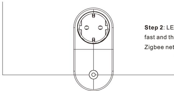
**Step 2:** LED indicator will flash white fast and the plug will try to join a Zigbee network.
