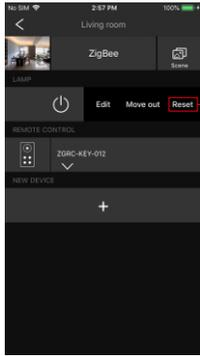
From your ZigBee controller or hub interface, choose to delete or reset the lighting device as instructed. LED indicator of the plug blinks white 3 times to indicate successful reset.
