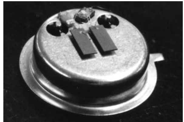
Fig. 2: Inside view of pyroelectric differential sensor with two air-suspended pyroelectric elements
