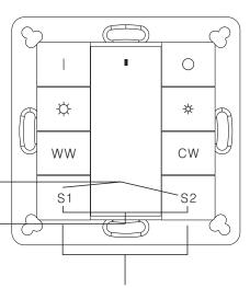
Network pairing mode: click both buttons 3 times to set the remote into network pairing mode (the remote should not belong to any gateway network).
